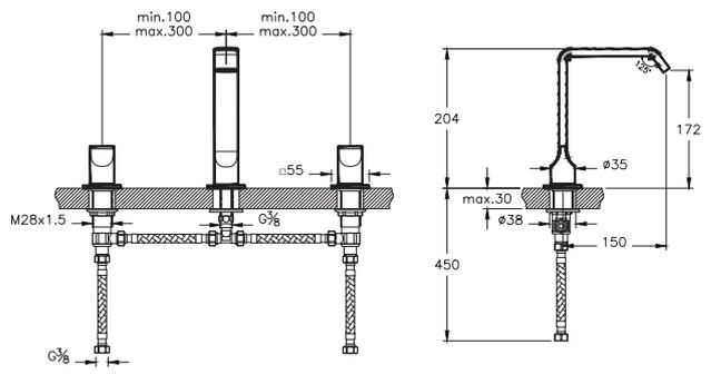
Technical drawings showing dimensions: min. 100, max. 300, min. 100, max. 300, 204, 172, max. 30, 150, 450, G<sup>3/8</sup>, M28x1.5, 55, 35, 38.
